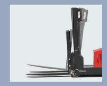
Mast tilting function is easy for entry in/out the nallet
