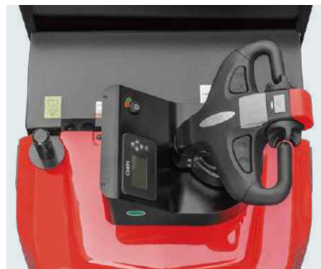
The dashboard with integrated large-screen instruments can be moved sideways to enable the changing battery easier
