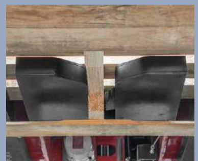
Manual-locking pallet clamp work on a wide range of pallets and accommodate pallet stringers ranging from 1" to 2" so operators can handle any pallet
