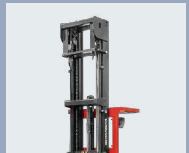
The mast chain with a safety factor of 10 times is equipped with a chain safety switch
