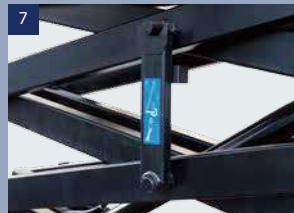
Supporting arms: To protect the operator when he is doing repair or maintenance job
