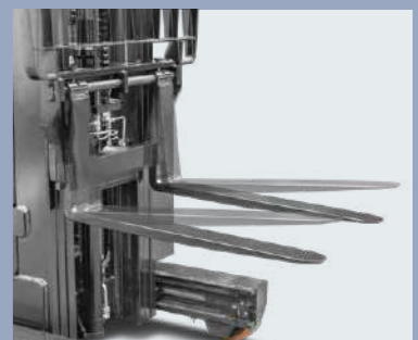
Forks can tilt forward/backward for easy loading
