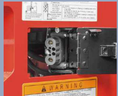
Charging plug inside operator's compartment, this eliminates the need to disconnect the plug from battery, enhancing ease of operation (Std.)
