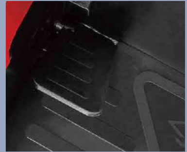
Safe pedal: when the pedal is released, traveling is stopped, and only hydraulic operation is enabled
