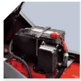
All the controllers, relays, and safety fuses are allocated in the controller box, free to water and dust. The main electronic components are waterproof, which is capable operater in severe environment. And the famous brand air-filter is also applied in the truck
