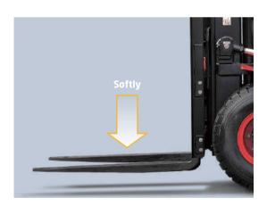
In addition to the soft landing system, the soft lifting system is adopted (front lifting cylinders of triplex mast and full free duplex mast), as a result, the noise and shock of the mast significantly decreases.
